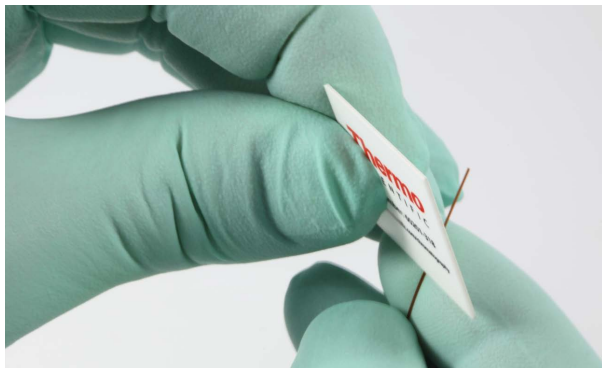
Figure 2: Cutting a fused silica column using a ceramic tile. For further details refer to the “GC Column Cutting Mini Guide” [1].
