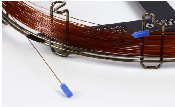
Figure 3: In this photo the front/inlet end of the column is on the right and wound on the top of the cage. The rear/detector end is seen on the left.
