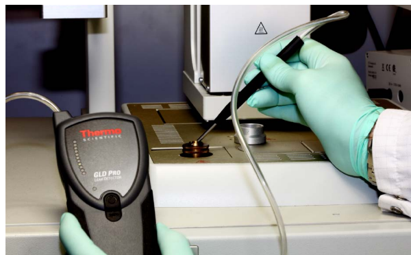
Figure 6: Thermo Scientific GLD Pro Gas Leak Detector (P/N 66002-001). Leak detectors such as this are highly sensitive and have a visual and audible alarm to signal when a gas leak is detected.
